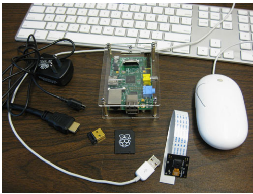
Fig. 2. Raspberry Pi camera system components. Pictured are the Raspberry Pi Model B in clear plastic case, PiNoIR camera, USB mouse and keyboard, micro-USB power adapter, HDMI cable, USB wireless Internet adapter, and SD card. [Color figure can be viewed at wileyonlinelibrary.com ]
