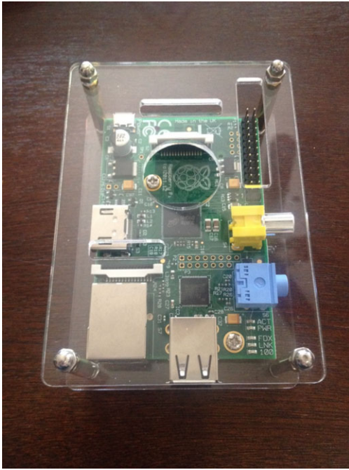
Fig. 1. The Raspberry Pi Model B in clear plastic case. [Color figure can be viewed at wileyonlinelibrary.com ]
