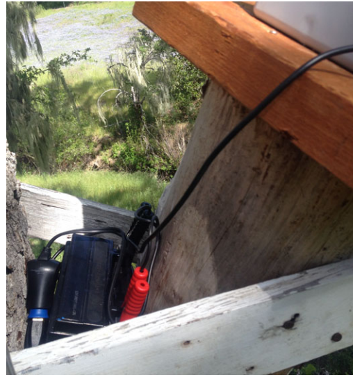
Fig. 6. Battery system without a waterproof plastic case. [Color figure can be viewed at wileyonlinelibrary.com ]
