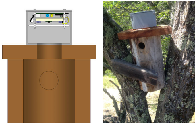
Fig. 4. Diagram and picture of an artificial woodpecker cavity with Raspberry Pi camera system installed in a weatherproof junction box on the cavity lid. [Color figure can be viewed at wileyonlinelibrary.com ]
